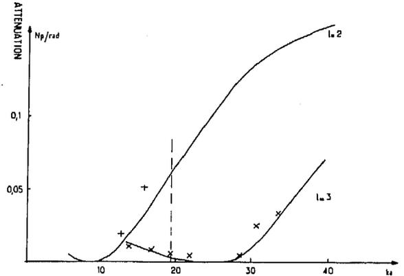
Fig. 3.1. — Attenuation of the Whispering Gallery waves  $l=2, 3$ . Solid curves: theory [7]; crosses: experiment [19].
