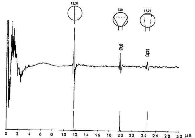
Fig. 3.2. — Experimental [12] and theoretical [9] arrival times of short sound pulses traversing a lucite cylinder (solid rays: dilatational; broken rays: shear).
