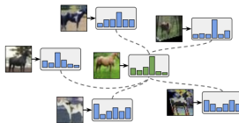
Figure 2: Augmentation anchoring. We use the prediction for a weakly augmented image (green, middle) as the target for predictions on strong augmentations of the same image (blue).
