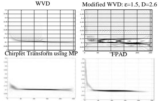
FIG. 8 : Comparative results for the hyperbolic chirp modulation
