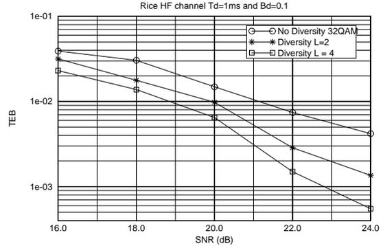
FIG. 3: BER of a  $L = 2$  and  $L = 4$  constellation, the CSI is given by a bilinear filter  $\eta = 3.75bit/s/Hz$ .
