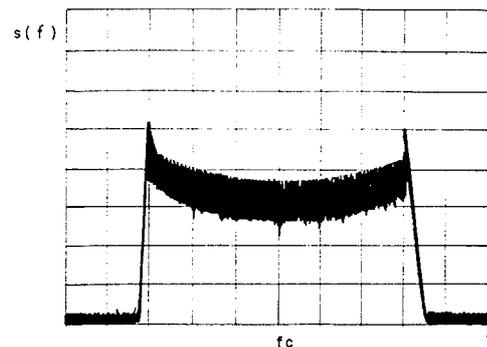
Figure 6: Probability density function of a sinusoidal signal, obtained using the spectrum analyser
