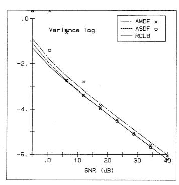
Figure 1: Variance of the DC TDE versus SNR compared to the Rao-Cramer Lower bound. The symbols x indicate simulation results (3000 runs).
