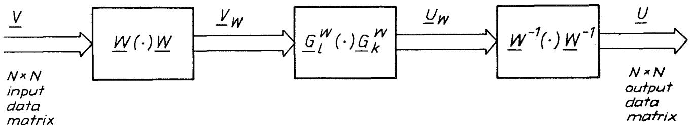
Fig.1. The block diagram of the Walsh domain restoration filter
