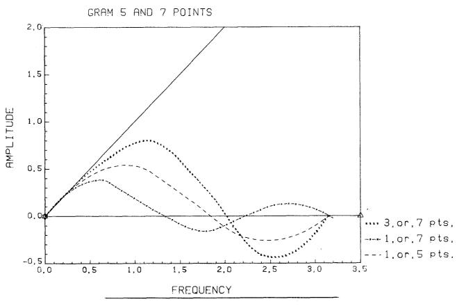
Digital filters for differentiating signals of low accuracy.
