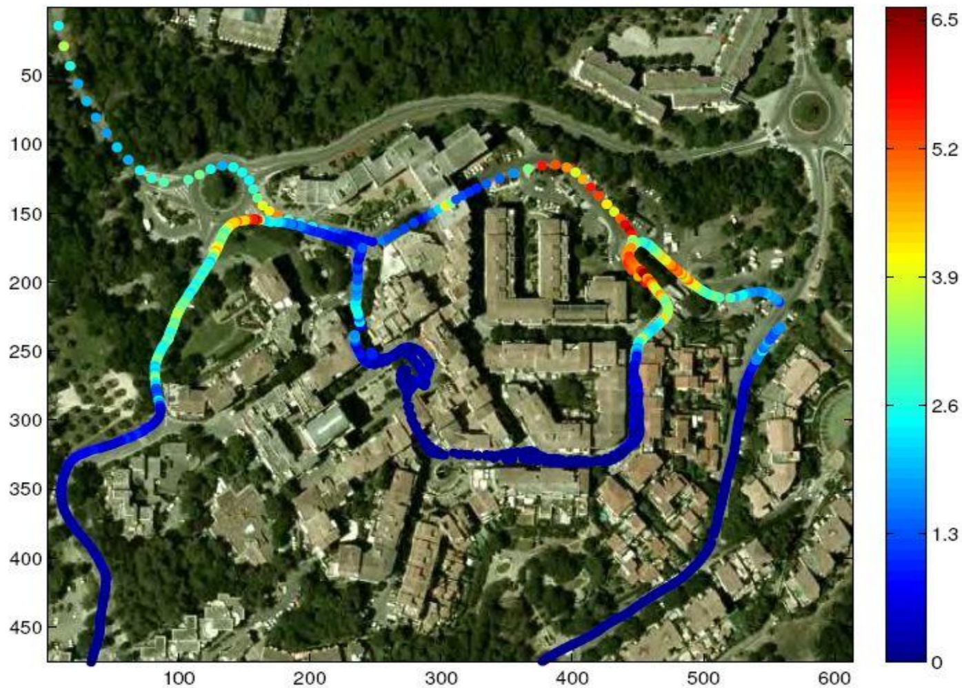
Figure 1.10: Mutual information of a 1x1 SISO system in an urban area for a SNR of 10 dB and constant transmit power.
