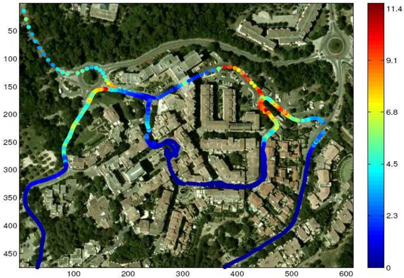
Figure 1.4: Mutual information of a 2x2 (dual polarized at the BS) MIMO system in an urban area for a SNR of 10 dB and constant transmit power.
