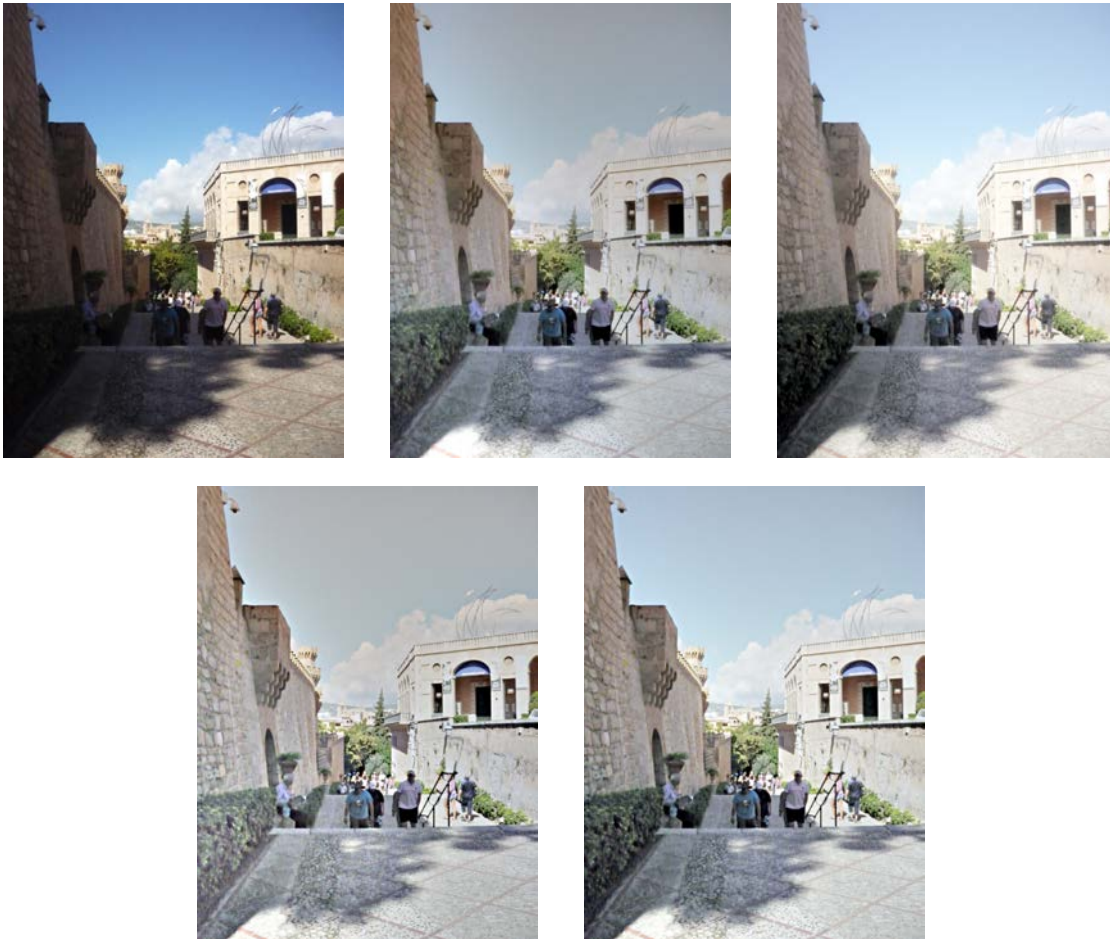
FIGURE 2 – An example of the role of the scales. Top left : Original image. Top center : Result of Single-Scale Retinex (SCR) with c_n = 250 . Top right : Result of SCR with c_n = 1000 . Bottom left : Result of Multi-Scale Retinex with c_0=15 , c_1=80 and c_2=250 , proposed values in article [6]. Bottom right : Result of Multi-Scale Retinex with c_0=15 , c_1=250 and c_2=1000 , values adapted to the size of the image.
