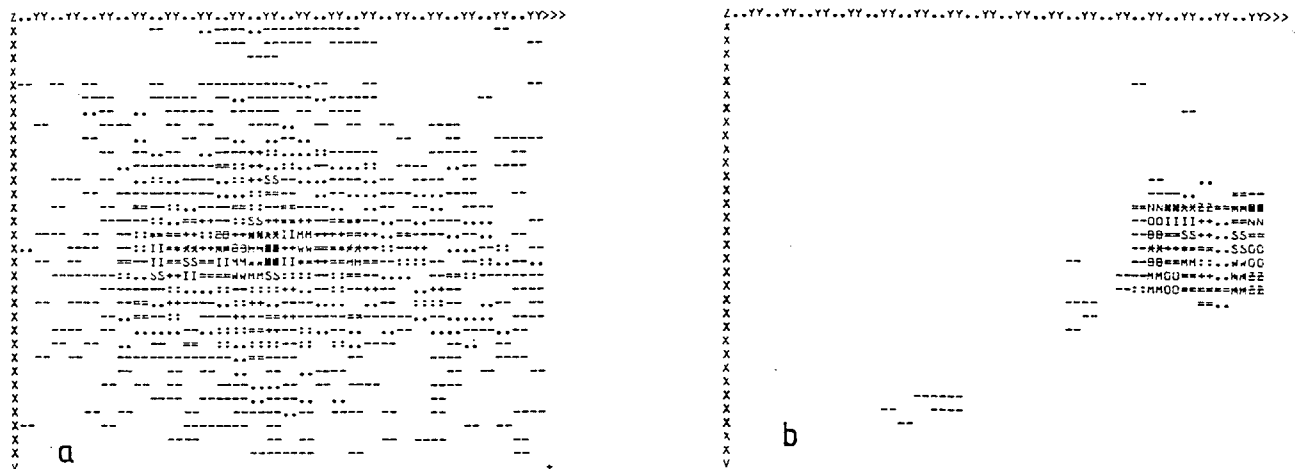
Fig. 4 Plexiglass plate ( \epsilon_r=2.5 ). a) Measured hologram. b) Image reconstruction from the measured hologram using equation (6). Data of the measuring equipment and for the reconstruction cf. Fig. 3.
